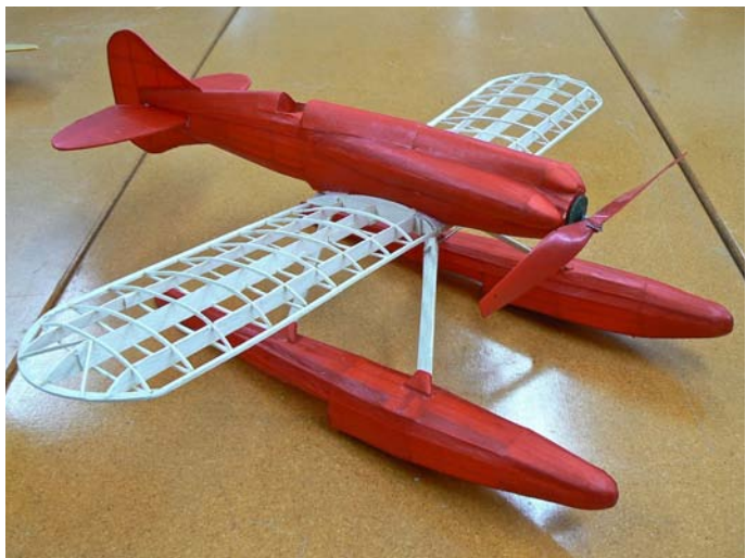
Left: Light wing construction is evident in George Fay's Macchi M67 Schneider Trophy racer.
